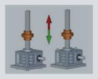
main load: tension upwards > support above
